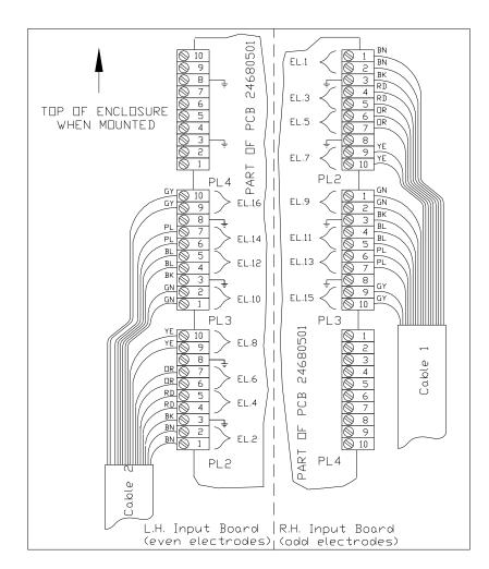
Figure 2.3: Enclosure cable layout for 16 electrode system
